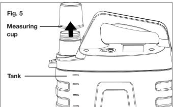
**3.** Fill the tank with the desired amount of water (up to 1 gallon).
